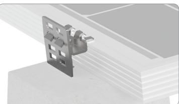
The special teeth of PowerClamp allow you to bite the frame of the PV modules, easily overcoming the anodized layer and ensuring a safe ground connection path of the system: all the panels are in fact connected in a single network through multiple connection points, and the earthing can be carried out quickly by placing a single ground lug per array.
