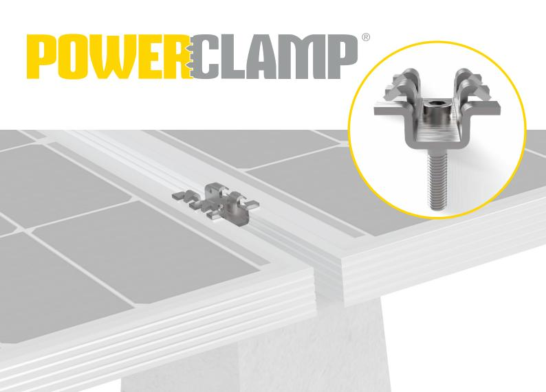
One accessory, double function: equipped with a simple and innovative design, the new Sun Ballast PowerClamp allows you to make photovoltaic systems even safer, both from an electrical and mechanical point of view. The special teeth ensures much easier, safer and faster grounding of the panels, while the top-quality stainless steel guarantees a solid and resistant clamping.
